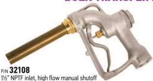
1½" NPTF inlet, high flow manual shutoff nozzle, has an aluminum body with brass valve stem, 1½" dia. x 8" long brass spout with Viton seals. Body includes "hold - open" notches. Ideal for use in dispensing oils, hydraulic fluids, antifreeze and diesel fuel. Weight 6 lb.
