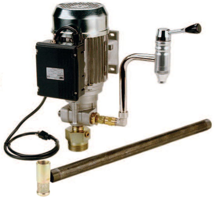
P/N 33221-S3 Vertical mount system includes 3.0 GPM electric pump, spigot, 2" double tap, 1"x30" suction pipe and foot valve. Ideal for use with 55 gallon drums and bench tanks.
