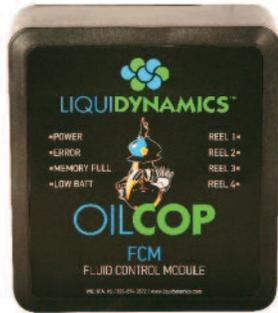
Each Fluid Command Module (FCM) includes a 115 VAC power module that is used to power the FCM as well as providing 24 volts to up to four Pulsar/Solenoid Modules (PSM's). The PSM's are quickly and easily connected to the Fluid Command Module (FCM) via a four conductor cable. This four conductor cable provides pulser/metering data to the Fluid Command Module (FCM) as well as power to the solenoids, thus simplifying connectivity immensely.
