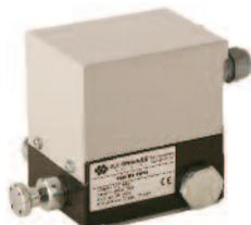
Pulser accuracy is +/- 0.5% with a maximum flow of 7.9 GPM and viscosity range of 9 – 3,000 cSt. Maximum operating pressure is 1,000 PSI, inlet filter/strainer is 150 micron.
