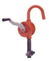
MODEL **MA-16**, P/N 10016 Heavy duty hand operated lever drum pump. with high volume output and hose thread fitting at discharge. Fits 16, 30 and 55 gallon drums. For use with light oils, ATF, 100% antifreeze, hydraulic fluids and diesel fuel. Includes telescoping suction pipe. Approx. 12 strokes/gal.
