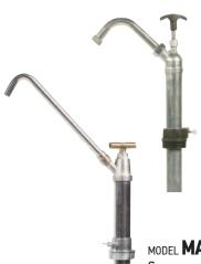
MODEL **MA-9**, P/N 10009 "T" Handle pump with curved "turn up" non drip spout. Includes 2" bung adapter suitable for 16 to 55 gallon drums. Typical uses include diesel fuel, light oils, ATF, antifreeze and other similar petroleum products. Approx. 1 stroke/qt.
