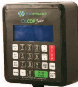
Additionally, the Junior Console stores up to 999 technician pin numbers and is used by the technicians to select which fluid to dispense, initiate dispensing operations such as preset dispense, manual dispense and top-off dispense.
