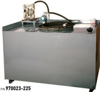
225 gallon bench tank with 3/4" double diaphragm pump and 4 way valve system can be used to evacuate portable oil drains in the suction valve position (fills the tank) and then the tank can be emptied by positioning the valve to the discharge position. System includes an air filter/regulator, 3/4" x 12' suction/ discharge hose with dry break disconnect, tank level gauge and lockable fill cap. The bench tank provides a convenient work surface in shops where space is a premium.
