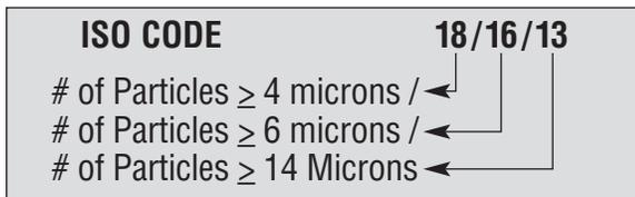
*Note: If the 4 micron particle count is not significant it will be replaced by an \*. i.e. \*/16/13*
