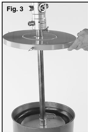
d. Loosen the wing nut securing the pump to the cover and allow the pump to slide to the bottom of drum, fig. 4, raise pump off the bottom slightly and tighten wing nut securing pump in position.
