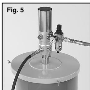
e. Attach any air inlet hoses/fittings and discharge hoses, fittings and accessories as required for your system, fig. 5.
