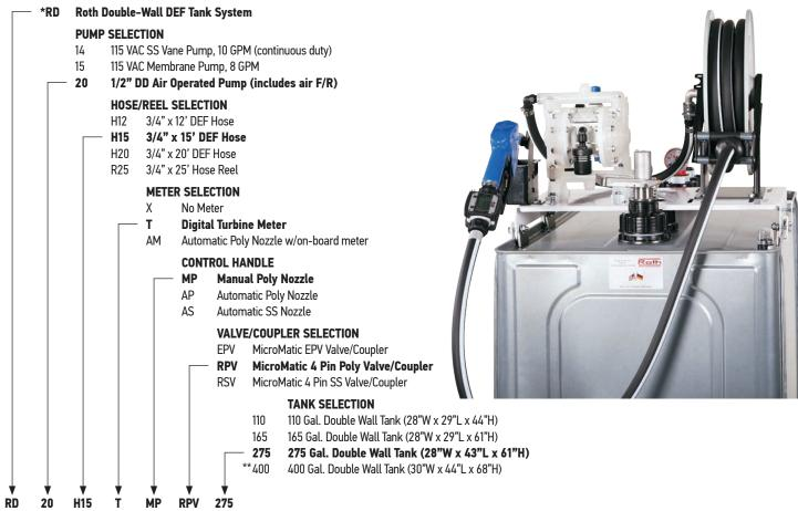
**Example:** Double Wall Roth Tank System with 1/2" double diaphragm pump, 15' hose, electronic digital turbine meter with quart calibration, Manual shutoff Poly nozzle, MicroMatic Poly RPV coupler and drum valve. System meets "Closed" system requirements according to ISO 22241 specifications. Tank selection in this case is the 275 Gal. double wall tank.
