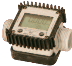
P/N 100388 DEF turbine pulse meter has a flow range of 1.5 – 26 GPM and working pressure up to 145 PSI. Fittings are 1" male BSPP and two each stainless steel adapters, 1" female BSPP x 1" female NPT are included.
