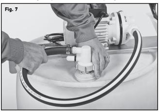
9. Place assembled Drum Topper kit onto top of drum as shown and secure in place with spring tension
